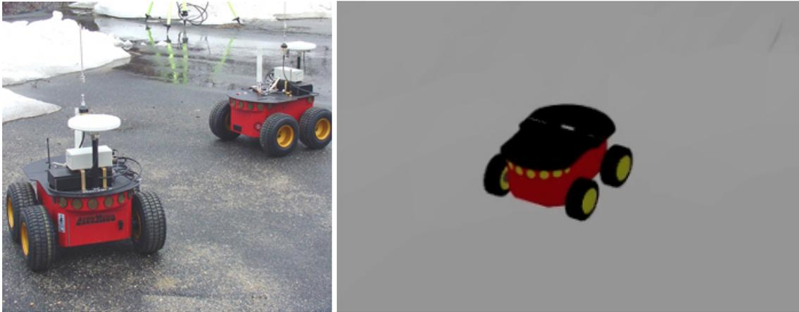
Figure 4.6: Pioneer 3at robots in use (left) (ROS-wiki, 2017) and rendered in Gazebo (right)
