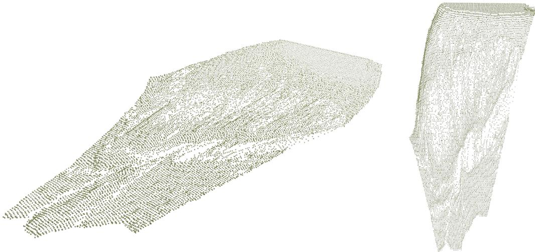
Figure 4.3: Terrain point cloud generated from a depth image
